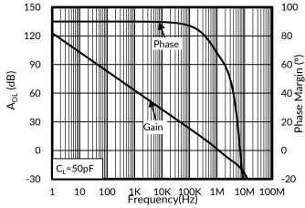
Figure 27. Open-Loop Gain and Phase vs Frequency
