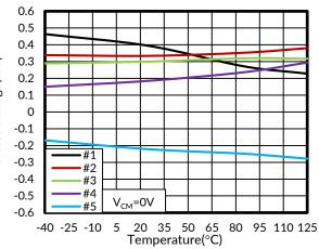
Figure 2. Offset Voltage vs Temperature
