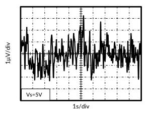
Figure 22. 0.1Hz to 10Hz Noise
