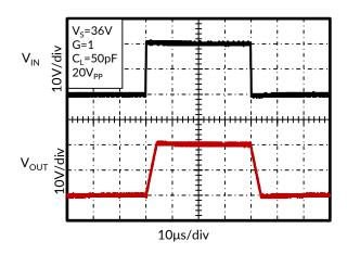
Figure 26. Large-Signal Step Response
