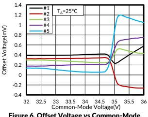
Figure 6. Offset Voltage vs Common-Mode Voltage (Transition Region)
