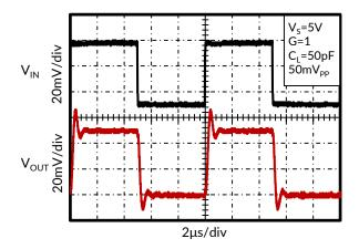
Figure 25. Small-Signal Step Response
