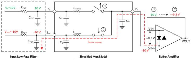
Figure 29. Back-to-Back Diodes Create Settling Issues
