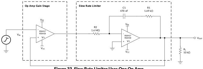
Figure 33. Slew Rate Limiter Uses One Op Amp
