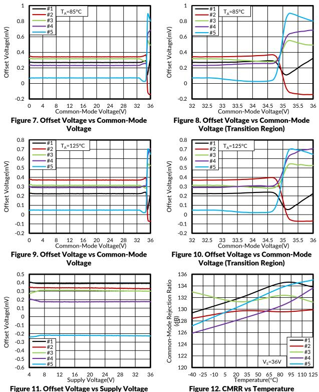
Figure 11. Offset Voltage vs Supply Voltage
