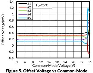
ure 5. Offset Voltage vs Common-N Voltage
