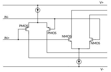
Figure 31. Rail-to-Rail Input Stage
