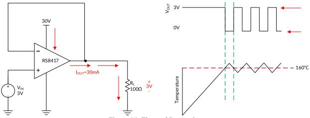
Figure 30. Thermal Protection
